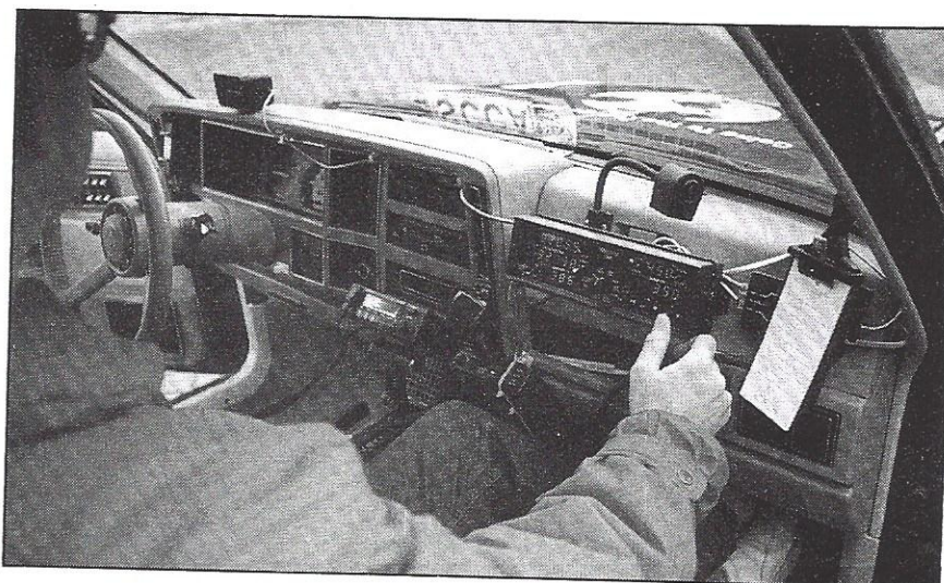
Jack's magic box—the Timewise mileage computer. Mileage can be adjusted accurately to 1/100,000th of an inch.
